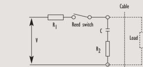
The above diagram illustrates a resistor/capacitor network for protecting a Reed Switch against high inrush currents. R<sub>1</sub> and/or R<sub>2</sub> are used depending upon circuit conditions.
