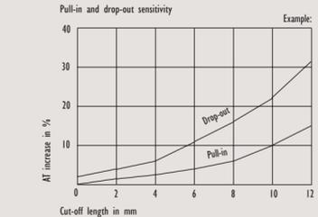
When cutting or bending Reed Switches, it is important that the glass body should not be damaged. Therefore, the cutting or bending point should be no closer than 3mm(.118) to the glass body.
